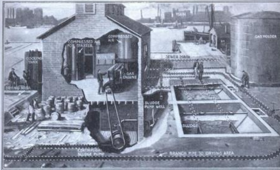
How the sewage disposal plant at Birmingham, England, supplies its own power is described in the illustration. Gas from the sewage drives an engine of 20 brake horsepower, which operates a centrifugal sludge pump.
